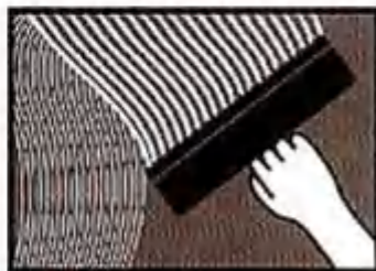
6 Tile Installation -Glue coating
