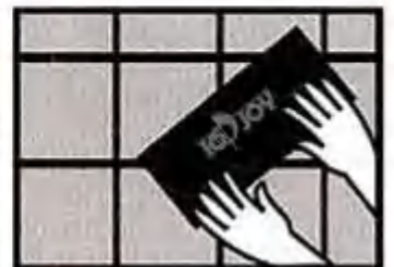
8 Tile Installation -Exhausting, roll pressing
