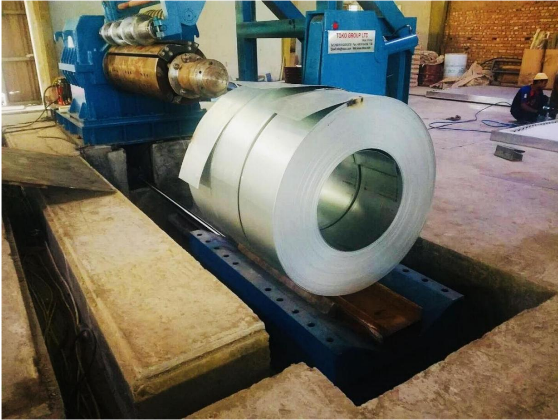
TOKO Slitting Line from Africa Customer's Factory
